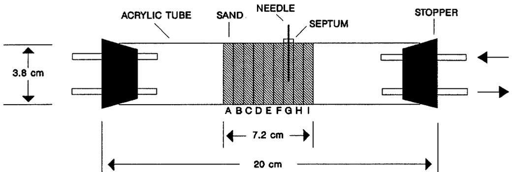
FIG. 1. Diagram of cylinder in which responses of nematodes to a point source of  $\text{CO}_2$  were studied.
