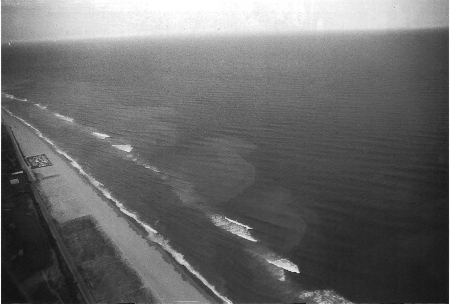
Rip currents near Barcelona, Spain. This oblique aerial photograph clearly shows the pattern of sediments suspended in the water column by near-shore rip currents. These sediment plumes are moved offshore in response to rip current action. (Photo: Alain Miossec. Taken April 2000.)
