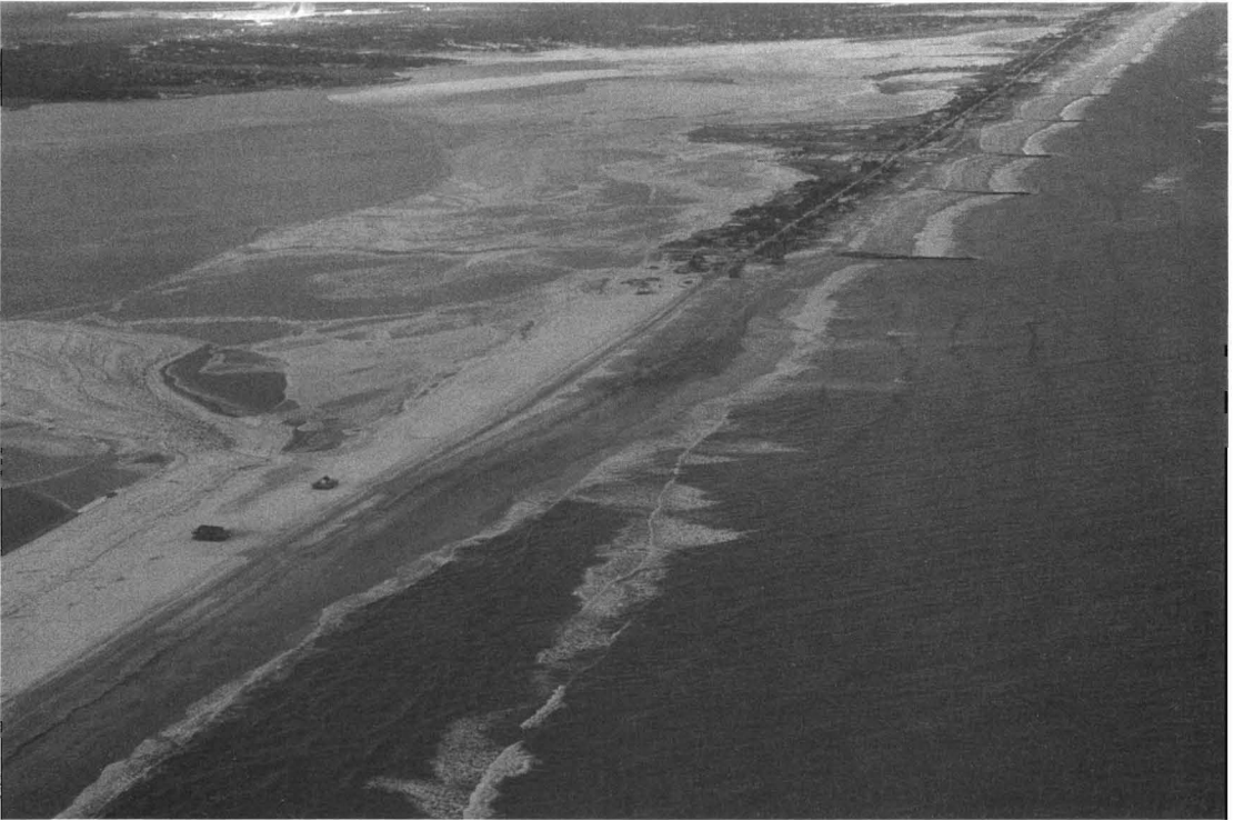
Little Pikes Inlet Fill Area, Westhampton, New York. Aerial photograph, view northeast, of the Little Pikes Inlet Fill Project, Westhampton, New York. The western end of the Westhampton Groin Field is pictured in the upper third of the photograph. Note that sand appears to be migrating from the offshore bar system into the nearshore surf zone. Further to the west, however, beyond the fill area erosion and flooding continues to be a problem with several houses lost in the last month. (Photograph by Dan Covello, 15 January 1994.)
