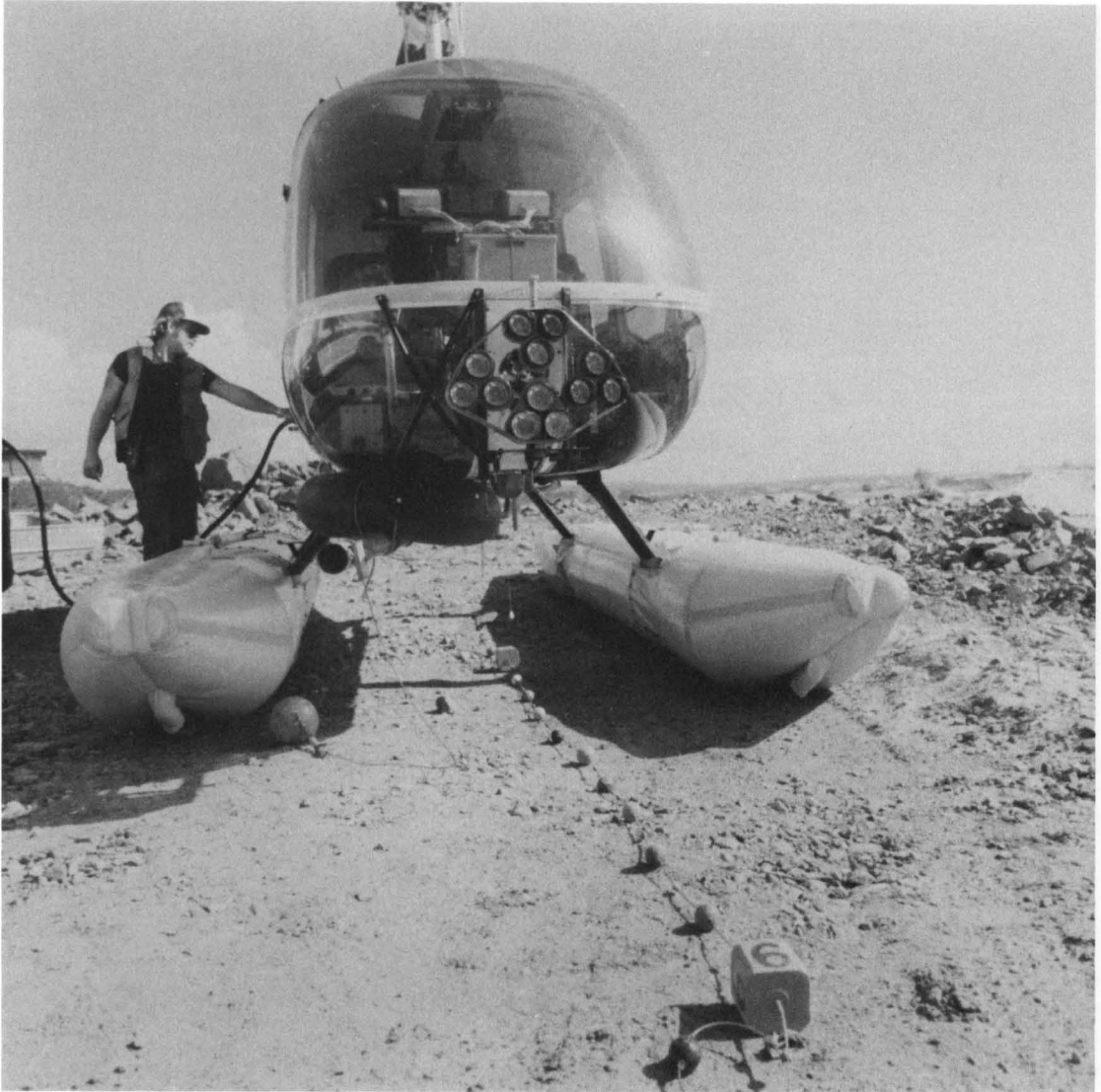
Figure 2. Helicopter, undercarriage, and survey cable.
