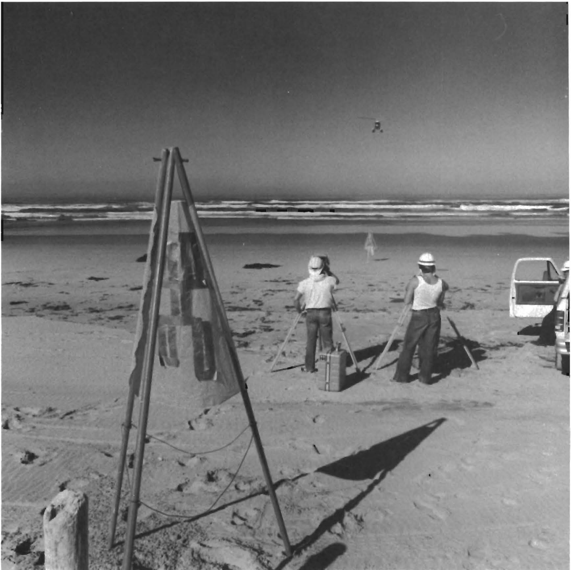
Figure 3. Helicopter, range poles, and total station on profile line.
