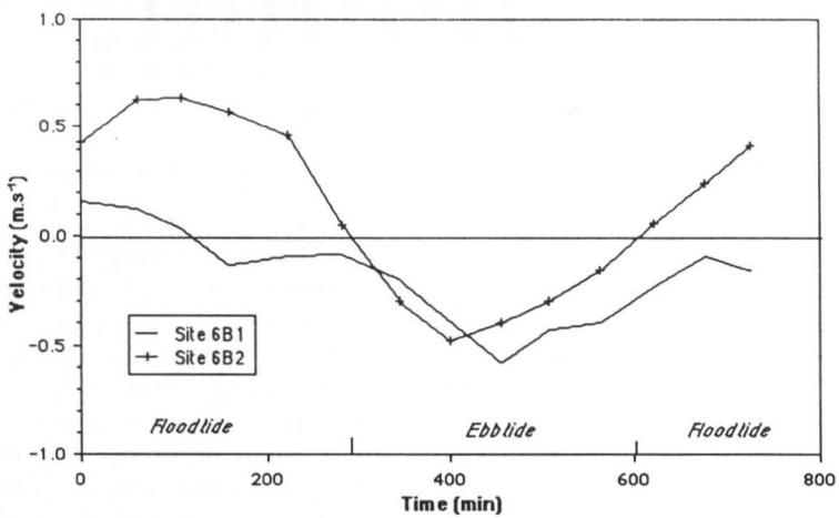
Figure 5. Time-velocity graph for Braystoke current measurements made in Cutter and Pilot Bay Channels during the THS (Figure 3). Ebb-directed flows are indicated by negative current velocities. The tidal flow within Cutter Channel is almost symmetrical, whereas the flow within Pilot Bay is strongly asymmetrical, indicating an ebb-dominance.
