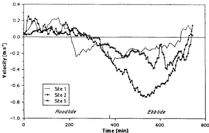
Figure 6. Time-velocity graph for the Aanderaa current meter measurements within Pilot Bay (locations given in Figure 3). Ebb-directed flows, which are indicated by negative current velocities, clearly predominate over the tidal cycle.
