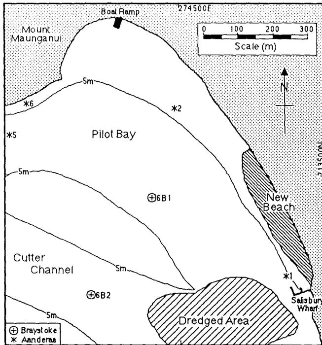
Figure 3. The sediment used to renourish Pilot Bay Beach was dredged from the junction of the Maunganui Roads, Cutter Channel, and Pilot Bay Channel, and piped to a discharge zone northwest of Salisbury Wharf. The locations of Anderaa and Braystoke Current monitoring sites are also indicated.
