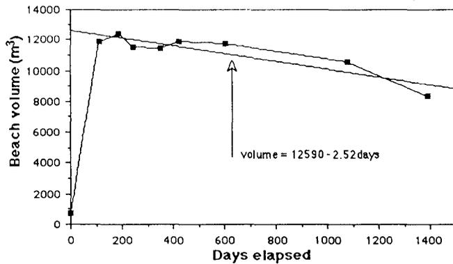
Figure 13. Beach volume above MLW (m<sup>3</sup>) for Pilot Bay Beach. The regression line shown predicts that all the sediment added during renourishment will be lost in 13 years.
