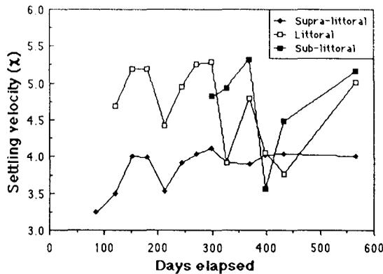
Figure 9. Temporal variations in the mean settling velocity ( $\chi$ ) observed within the highly variable zone of Pilot Bay Beach. Increases in mean settling velocity (indicating a decrease in apparent grain size) occurred after storms and were associated with an influx of low density pumiceous clasts.
