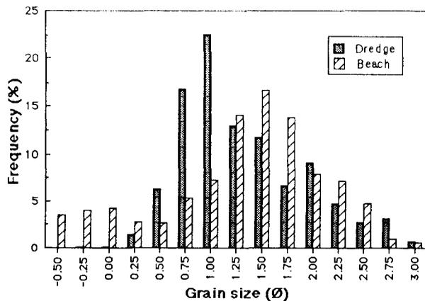
Figure 7. Particle size distributions for the pre-nourishment surficial sediments (average of 11 sites) and the dredge spoil (average of 3 sites).
