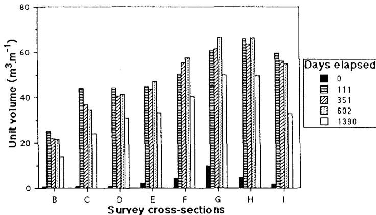
Figure 12. Unit volumes ( $\text{m}^3 \cdot \text{m}^{-1}$ ) above mean high water for Pilot Bay Beach corresponding to the surveys in Figure 11.
