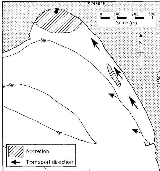
Figure 14. Summary of the sediment transport pathways for the renourishment sediment, and the major zones of sediment accumulation during the period April 1984 to October 1987.
