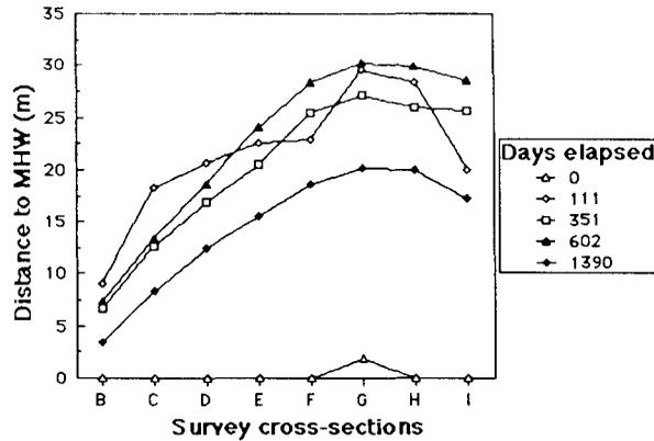
Figure 11. Distance to the mean high water elevation from the location of the gabion basket seawall for Pilot Bay Beach. The initial survey (day 0) was performed on December 16, 1983, and the first survey after renourishment (day 111) was performed on April 4, 1984.
