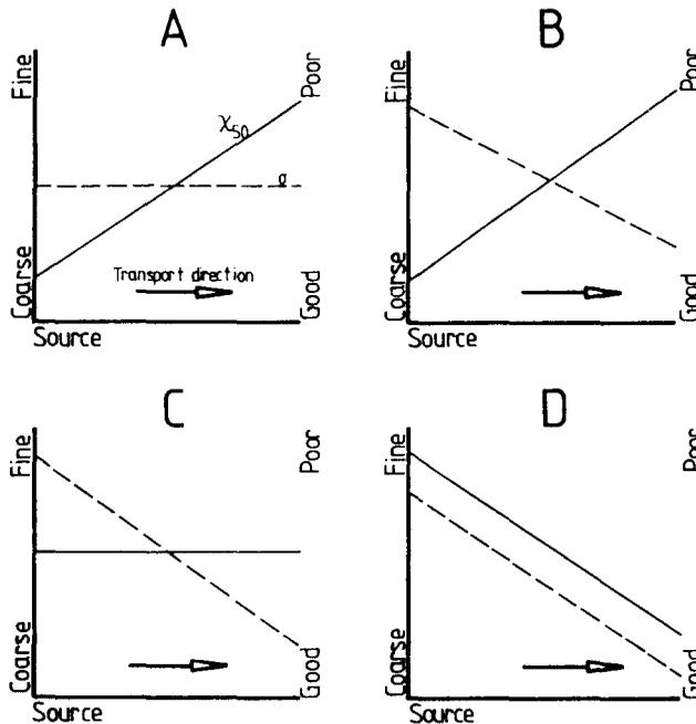
Figure 10. Spatial trends of median settling velocity and sorting which are considered significant in terms of defining sediment transport directions (After Sunamura and Horikawa (1972)). **A** indicates a progressive fining of the sediment with no change in sorting; **B** indicates a fining in sediment with improved sorting; **C** indicates no change in mean grain size with an improvement in the sorting; and **D** indicates a coarsening of the sediment with an improvement in sorting.
