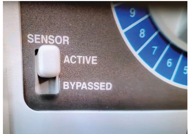
Figure 5. Irrigation controller with the sensor switch on the “Active” position.
