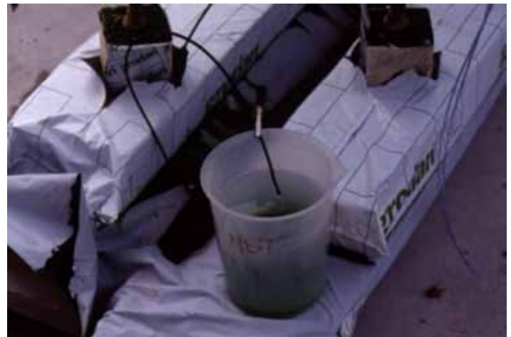
Figure 25. Collecting nutrient solution in a bucket from an extra emitter to track solution delivery rate and amount.
