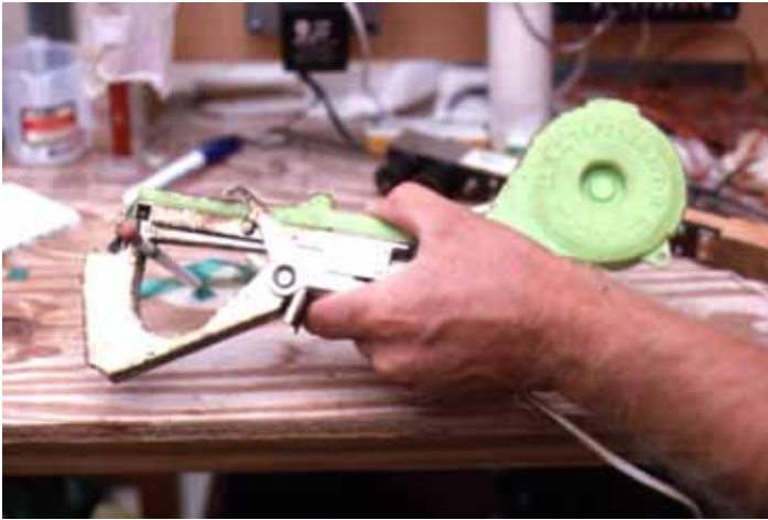
Figure 17. The “tapener” fastener for attaching the plant stem to the trellis string.
