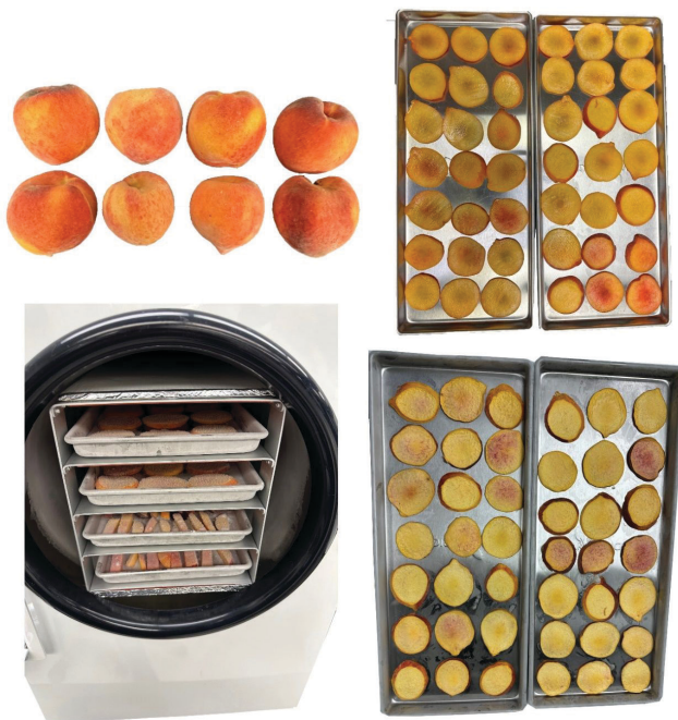
Figure 10. The steps and process of freeze-drying 'UFOne' peach. (Top left) Fresh fruit, (top right) fresh peach slices, (bottom left) freeze-drying process, and (bottom right) freeze-dried peach slices. Credits: Fariborz Habibi and Ali Sarkhosh, UF/IFAS
