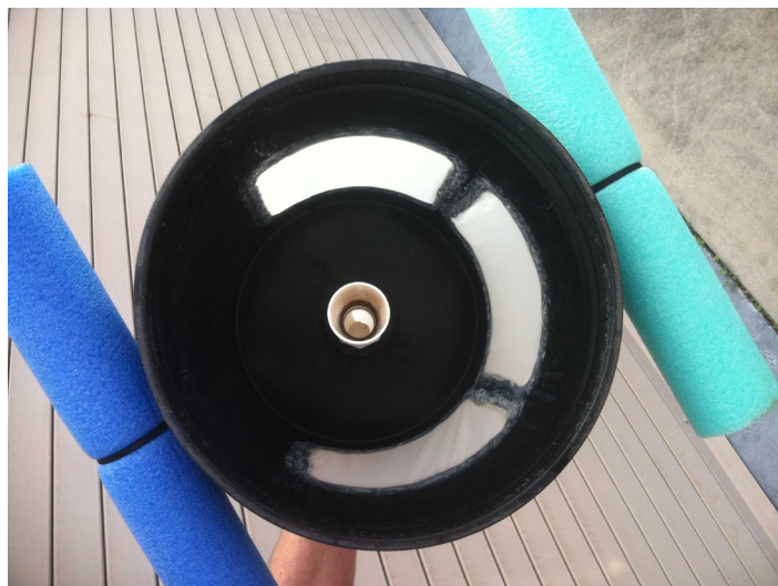
Figure 2. An internal view of the collection bucket portion of a floating airlift collector used at the University of Florida's Tropical Aquaculture Laboratory. Credit: Jason S. Broach
