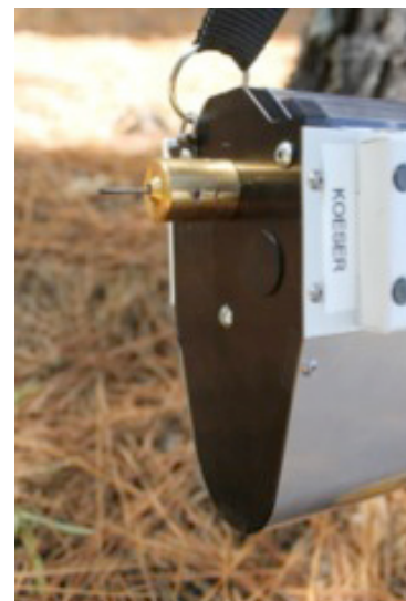
Figure 2. Close up of the drilling needle and the needle sleeve. Credits: Gitta Hasing
