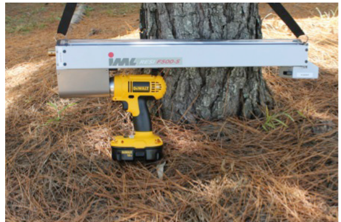
Figure 1. IML Resistograph® model F500-S. Credits: Gitta Hasing
