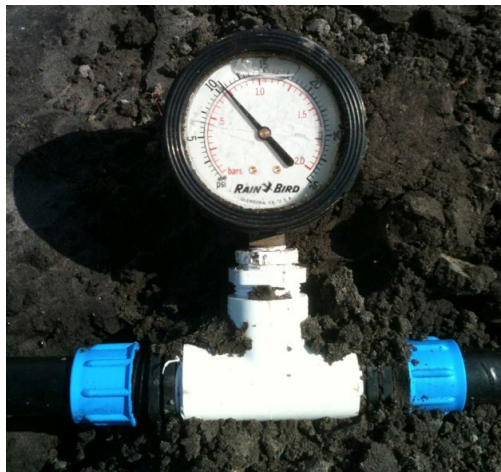
Figure 4. Water pressure gauge installed in-line in the drip tape over 1,300 ft from the irrigation manifold showing a pressure greater than 10 psi.
