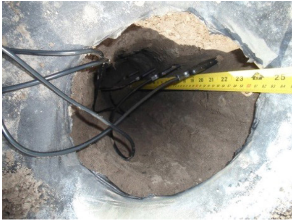
Figure 5. Top view of soil moisture sensors installed under plastic mulch at 4", 8", 16", and 24" depths.
