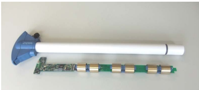
Figure 1. EasyAg multi-sensor probe with sensors (bottom) at 4, 8, and 12 inches. The PVC pipe (top) is the access tube (1.2 inch diameter) that houses the probe. The probe can be connected to a wireless datalogger and transmit the data to the farm office for its use or be made available on the Internet for it to be accessed by anyone. Credits: http://www.sentek.com.au
