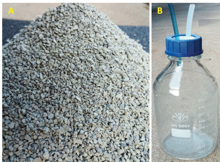
Figure 5. A) Grouting bentonite used as a sealant. B) Sampling bottle used to collect soil solution.
