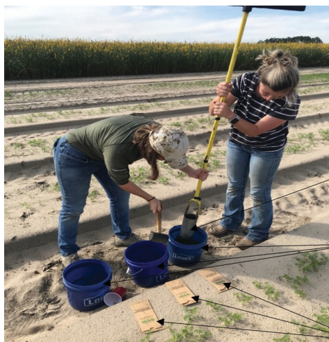
Figure 2. Soil sampling at different depths using soil auger in carrot production system.
