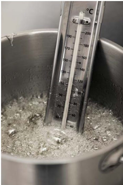
Figure 6. Several types of thermometers are available. Look in the kitchen appliance section for a waterproof thermometer with a probe to place in the water to test the temperature.
