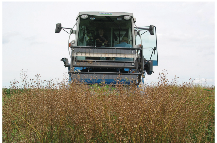
Figure 6B. Harvesting camelina with a grain combine. Credits: David Wright, UF/IFAS
