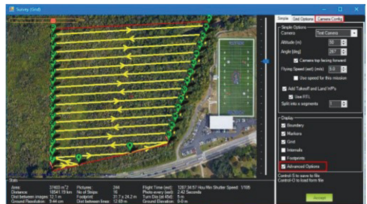
Figure 11. Example generated survey flight path. Credits: J. Chintanadilok, UF Department of Computer Science and Engineering
