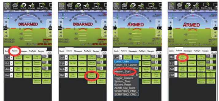
Figure 14. Menu buttons to arm the drone and begin the mission. Credits: J. Chintanadilok, UF Department of Computer Science and Engineering
