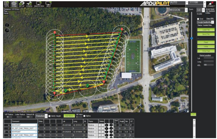
Figure 13. Fully generated Survey flight path generated in a polygon adjusted for camera settings. Credits: J. Chintanadilok, UF Department of Computer Science and Engineering
