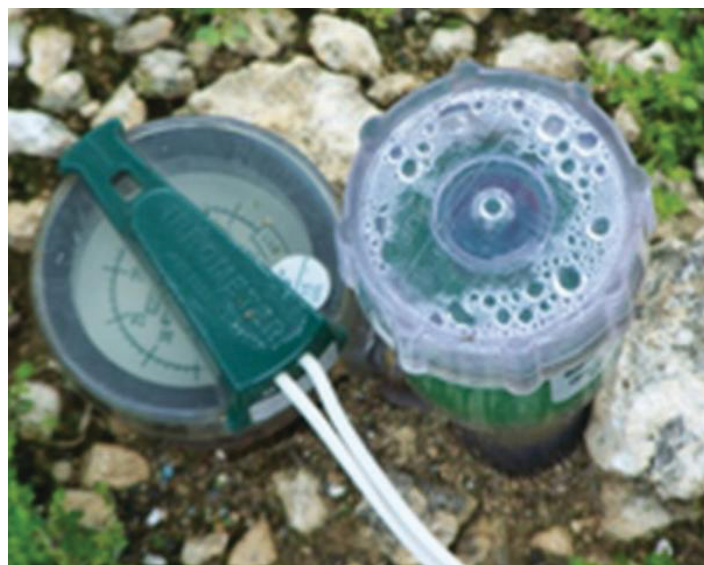
Figure 4. Tensiometer installed in very gravelly loam soil.
