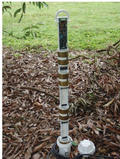
Figure 5. Multi-sensor capacitance probe being inserted into a field. Credits: Luis Barquin
