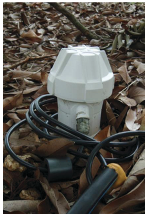
Figure 6. Multi-sensor capacitance probe installed in a south Florida grove. Credits: Luis Barquin
