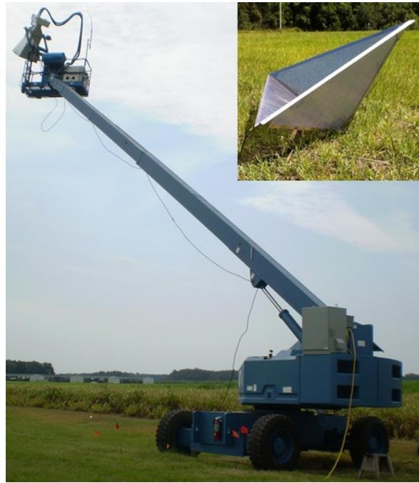
Figure 9. UF-LARS mounted on the 25 m Genie platform. (Inset) Trihedral calibration target made of aluminum with an aperture length of 1.28 m.
