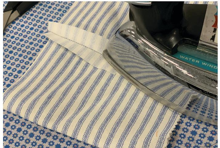
Figure 4. Pressing a seam.
