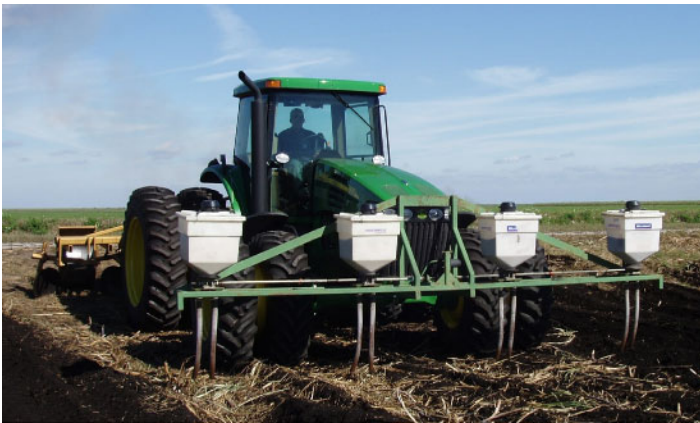
Figure 2. Application of granular insecticide for control of wireworms at sugarcane planting. Credits: Ron Cherry
