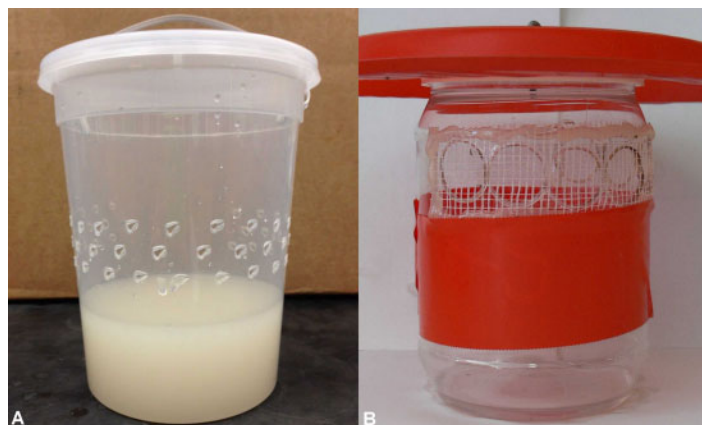
Figure 3. a) 32-oz clear plastic cup trap baited with yeast sugar water and b) 32-oz jar with red tape and large holes covered with drywall mesh.
