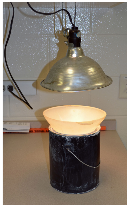
Figure 25. Homemade light trap for collecting insects. Credits: Robert Leckel, University of Florida
