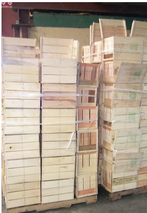
Figure 4. Wooden wirebound produce containers (1 1/9 bushel). Credits: Mark Ritenour
