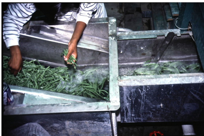
Figure 11. Snap beans being sorted upon exit from a hydrocooling flume.
