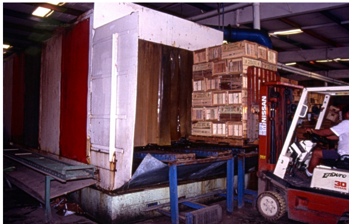
Figure 12. Cooling sweetcorn in a shower hydrocooler.
