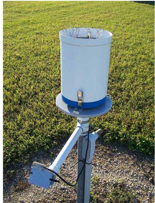
Figure 1. Tipping bucket rain gauge.
