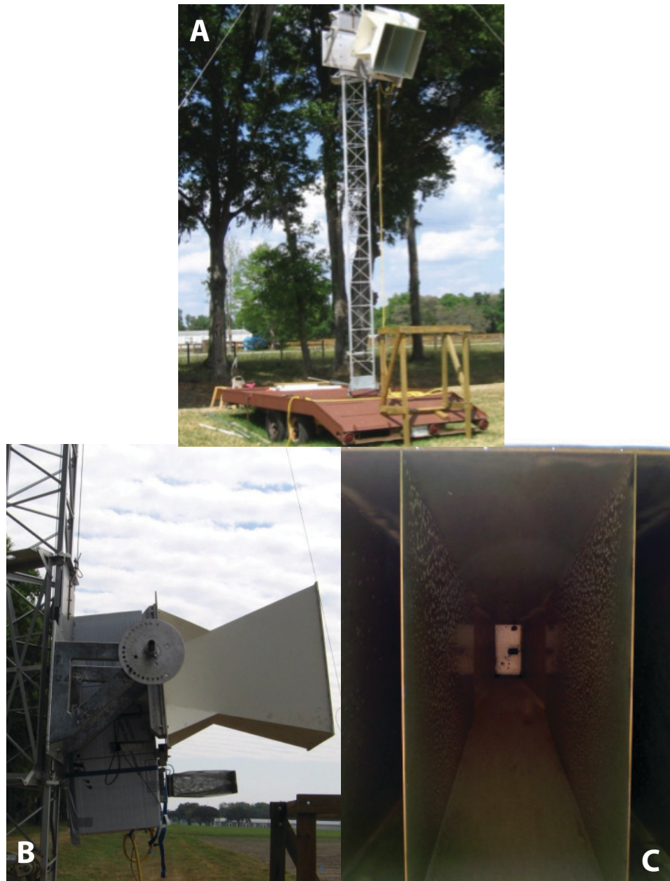
Figure 6 (a) The UFLMR system, (b) the side view of the UFLMR showing the rotary system, and (c) the front view of the UFLMR showing the receiver antenna.
