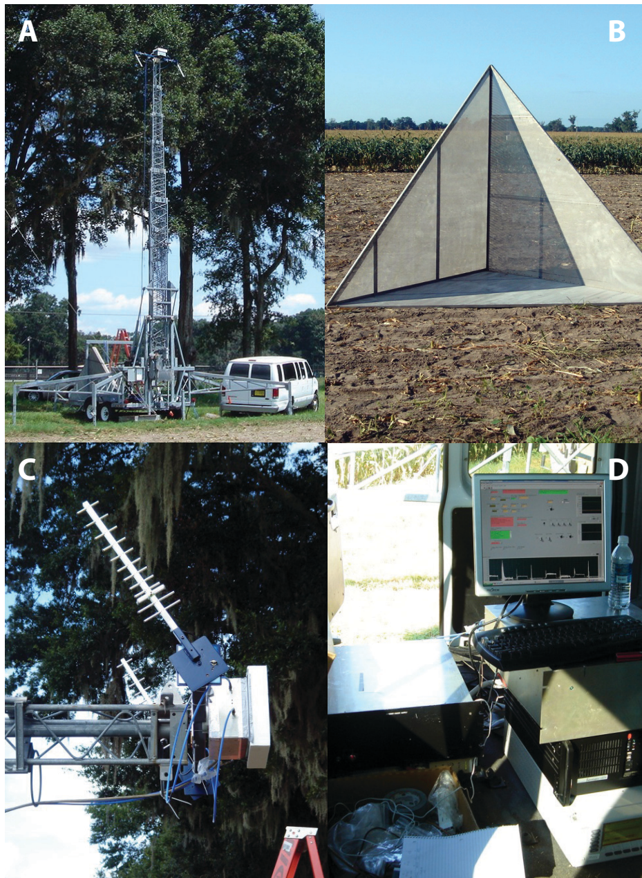
Figure 8 (a) The MOSS system, (b) corner reflector, (c) antennae and tower-mounted electronics, and (d) ground-mounted electronics.
