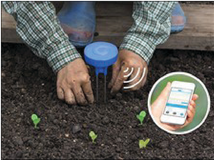
Figure 1. Sensoterra soil moisture sensors ( www.sensoterra.com ) from the Netherlands. Credits: Sensoterra
