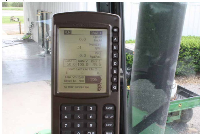
Figure 4. An applicator can use the monitor inside a self-propelled sprayer to adjust pressure and speed.
