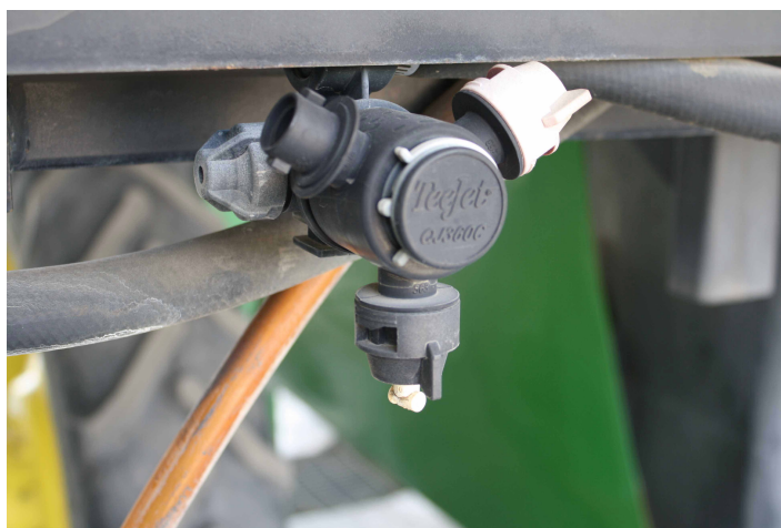
Figure 2. A nozzle includes the nozzle body, strainer, core, disc, and nozzle cap.
