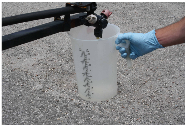
Figure 3. An applicator performs the nozzle flow test. Credits: Michael R. Miller
