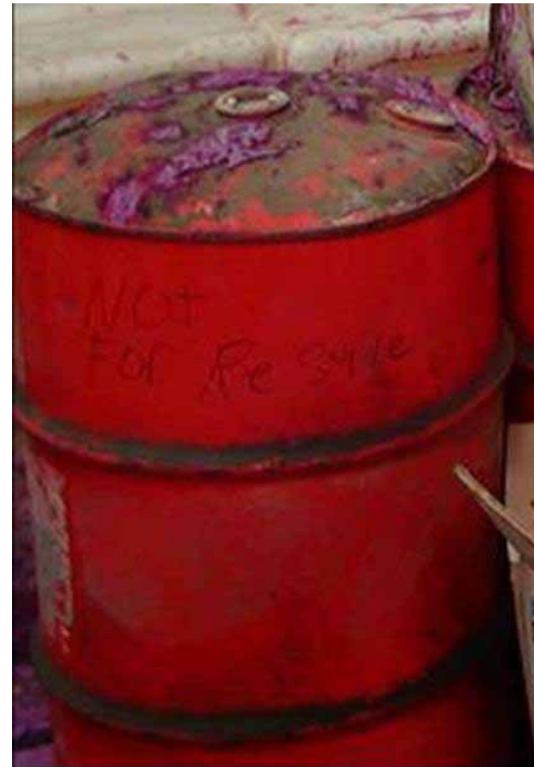
Figure 1. Pesticide drum bulging from extreme heat.
