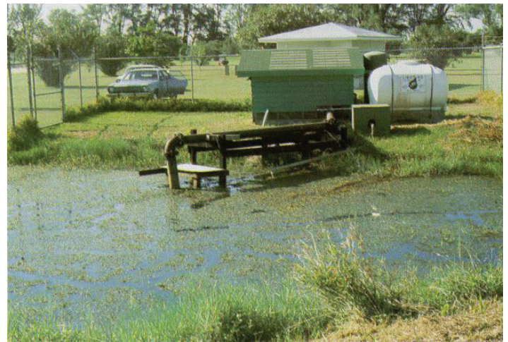
Figure 1. Dense Hydrilla growth can seriously impact agricultural operations, shown here blocking the intake line of an irrigation pump. Credits: David L. Sutton
