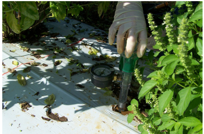
Figure 12. Placing tensiometer into hole with slurry. Credits: Kati Migliaccio
