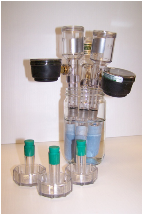
Figure 3. Soaking tensiometers in clean water overnight. Credits: Tina Dispenza
