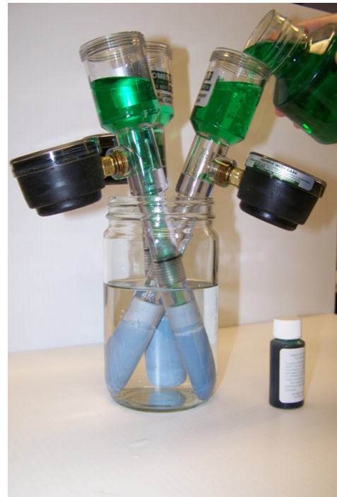
Figure 4. Filling tensiometers with water mixed with biocide. Credits: Tina Dispenza
