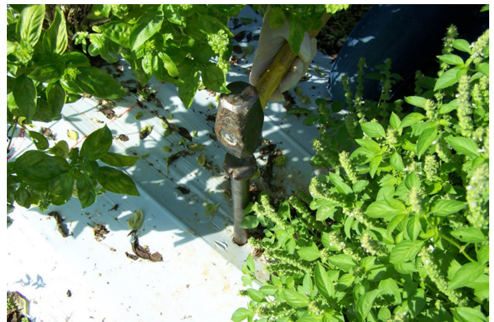
Figure 8. Hammering in the rod to make a hole for the tensiometer. Credits: Kati Migliaccio
