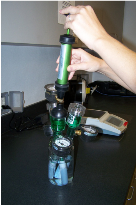
Figure 6. Applying pressure using a handheld vacuum pump. Credits: Tina Dispenza
