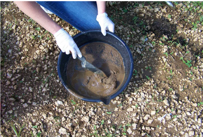
Figure 10. Mixing the sieved soil with water to make a slurry. Credits: Kati Migliaccio
