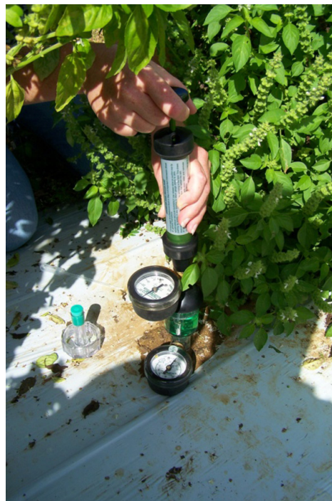
Figure 14. Servicing tensiometer in the field; applying pressure with vacuum pump. Credits: Tina Dispenza
