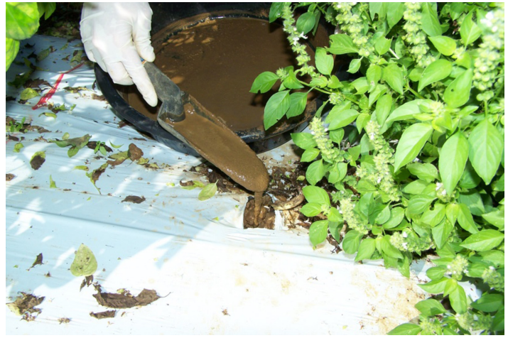
Figure 11. Pouring slurry into the tensiometer hole. Credits: Kati Migliaccio
