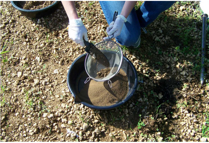
Figure 9. Sieving soil for making the slurry. Credits: Kati Migliaccio
