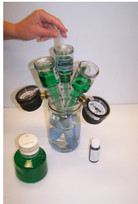
Figure 5. Checking for air bubbles trapped in the tensiometer column. Credits: Tina Dispenza
