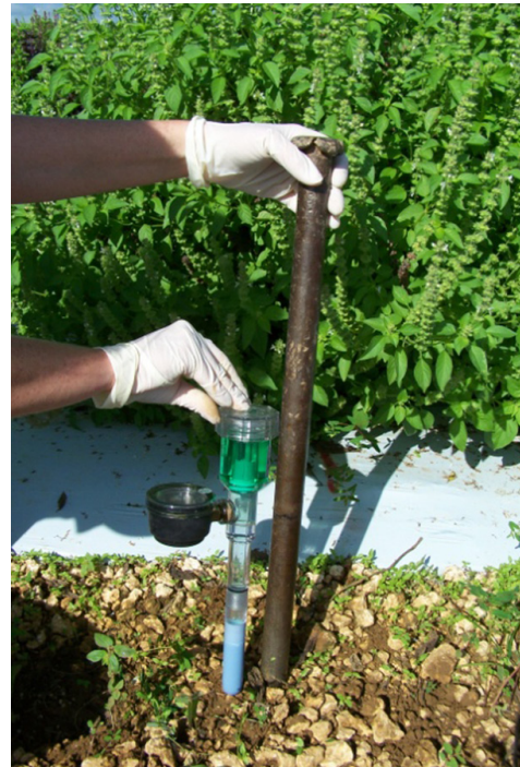
Figure 7. Rod used to make hole for tensiometer installation in the field. Credits: Kati Migliaccio
