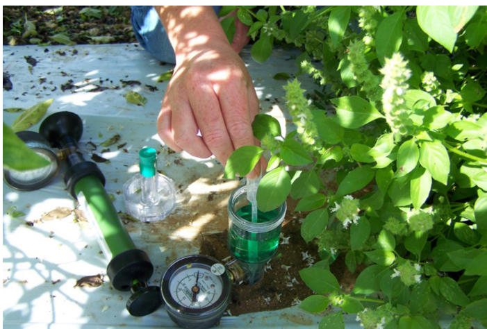
Figure 13. Servicing a tensiometer in the field; purging bubbles from water column. Credits: Tina Dispenza
