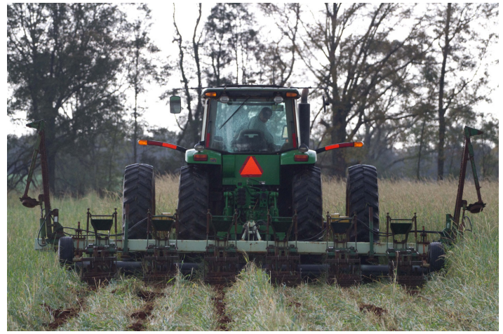
Figure 2. Custom roller/strip-till implement by Myron Johnson of Headland, Alabama. Credits: Brian Kahn
