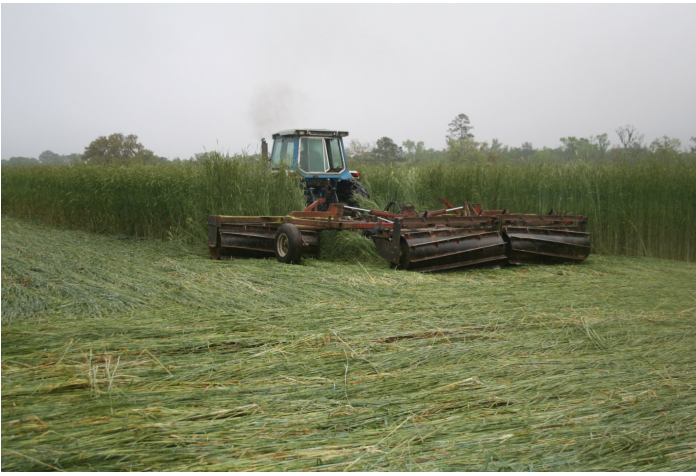
Figure 1. Cereal rye cover crop rolling/crimping in late March 2011 at Brock Farm in Monticello, Florida. Custom roller/crimper design and fabrication by Kirk Brock. Credits: Danielle Treadwell
