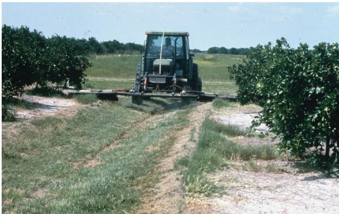
Figure 4. Boom applicator used to apply suspension fertilizers.
