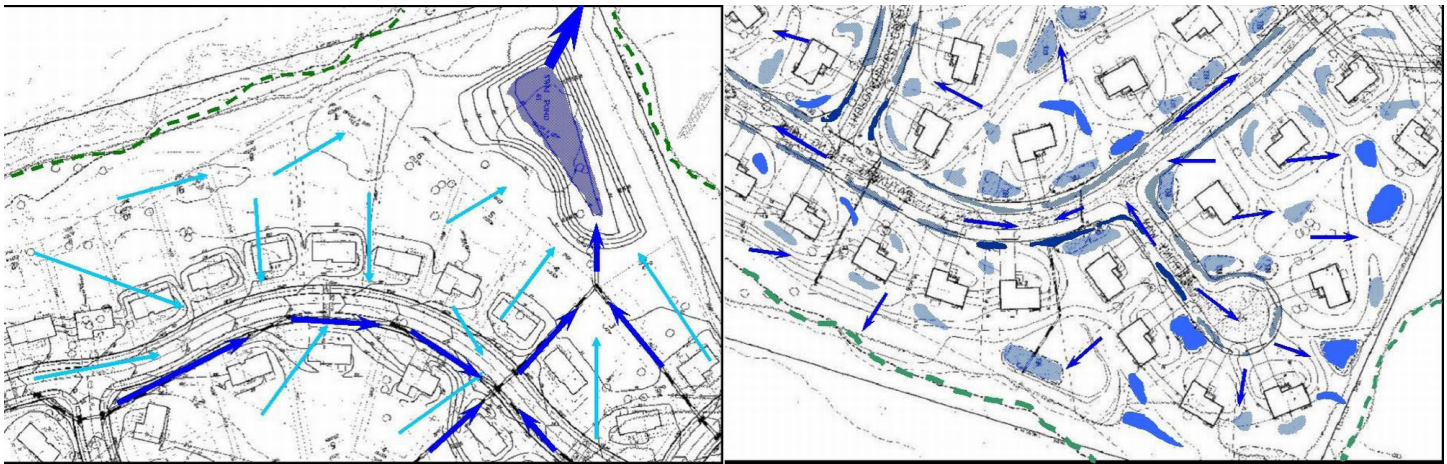
Figure 1. Centralized (left) stormwater management scheme vs. decentralized (right), “LID” scheme. Credits: Prince George’s County, n.d.
