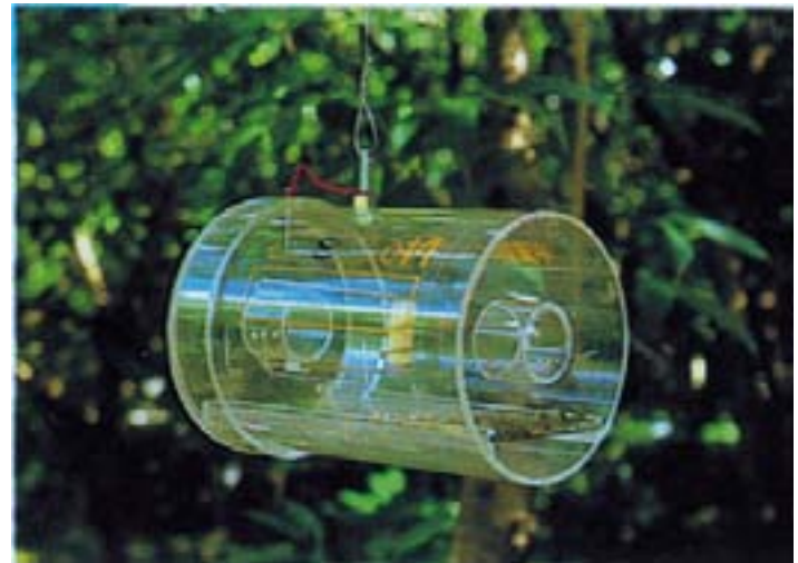
Figure 15. Steiner trap used to monitor and control the oriental fruit fly, Bactrocera dorsalis (Hendel).
