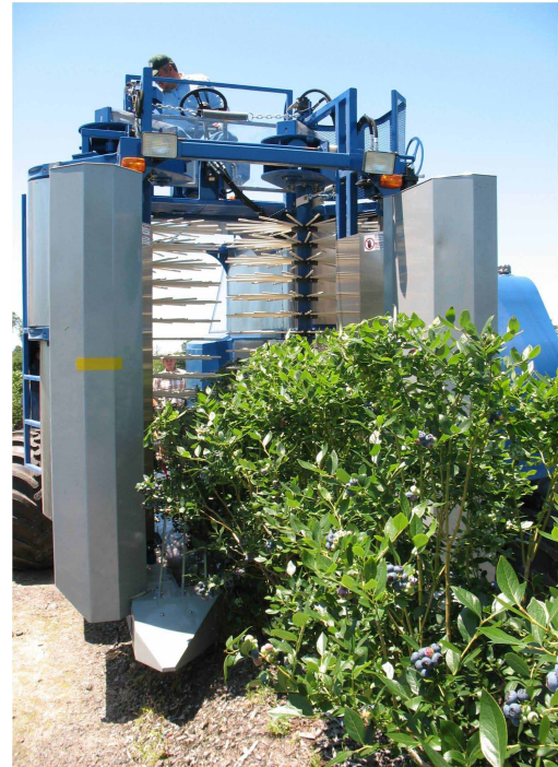
Figure 5. Mechanized harvest of southern highbush blueberry
