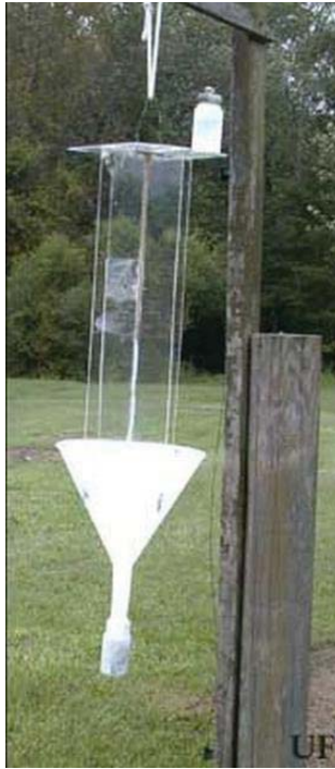
Figure 7. Emerging granulate ambrosia beetles, Xylosandrus crassiusculus (Motschulsky), can be trapped using an ethyl alcohol bait trap. Photograph by: R.F. Mizell, University of Florida.
