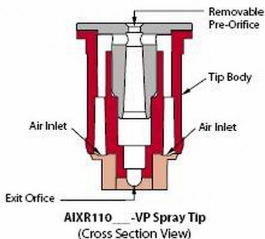
**Figure 8.** Cross section view of an air-induction nozzle. Credit: Spraying Systems Co.
