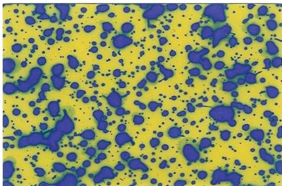
**Figure 10.** Droplets produced from an air-induction nozzle. Credit: J. A. Ferrell, UF/IFAS Dept of Agronomy.
