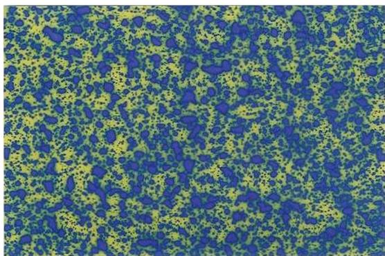
**Figure 11.** Droplets produced from a standard flat fan nozzle. Credit: J. A. Ferrell, UF/IFAS Dept of Agronomy.
