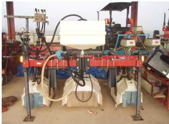
**Figure 15.** Shielded spray boom. Credit: UF/IFAS Pesticide Information Office.
