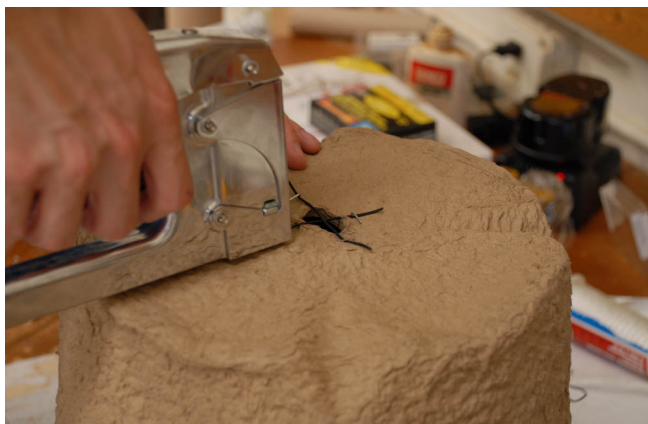
Figure 3. Staple two pieces of wire in the shape of a cross across small trap opening. Credits: M.K. O'Malley, University of Florida
