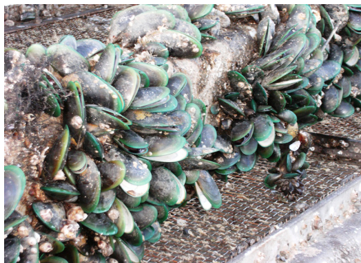
Figure 6. Filter from a power plant fouled with green mussels. Credits: Tammy Hatfield, Pelotes Island Nature Preserve, Jacksonville Credits:
