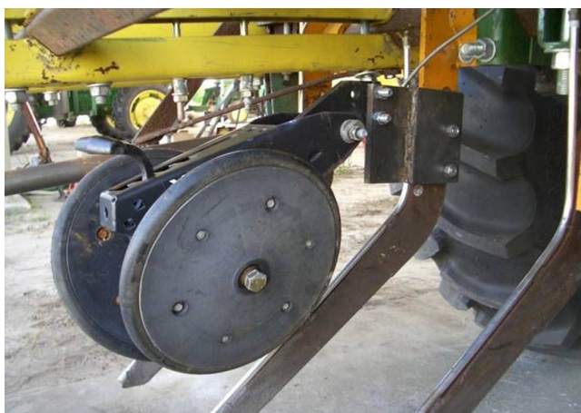
Figure 7. Modified rig for closing chisel marks.
