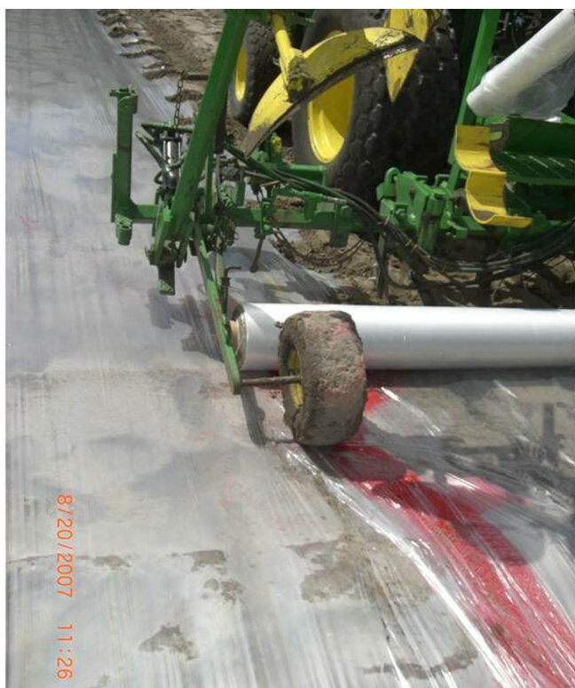
Figure 4. Gluing LDPE is currently standard for broadcast fumigation. Gluing VIF is problematic because of the need for plastic to be permeable to oxygen for the glue to cure.
