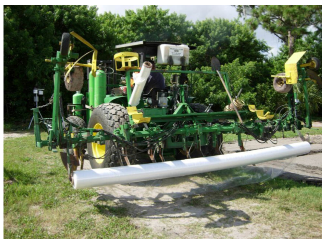
Figure 2. Wide plastic is needed (13 ft wide) for broadcast flat fumigation.
