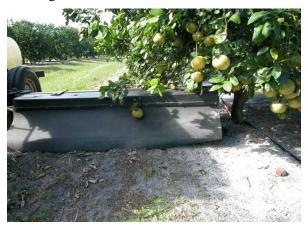
Boom placement. The herbicide boom should be far enough below the tree canopy to avoid fruit damage. The boom must be high enough for the weeds to pass under and be sprayed by the herbicide. Credits: UF/IFAS
