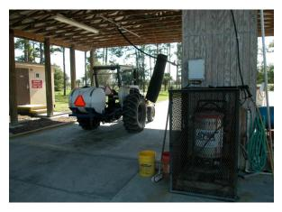
**Clean up.** After an application, the equipment needs to be cleaned up. Facilities like the one above are designed with sloped floors and tanks for capturing rinsate. Credits: UF/IFAS
