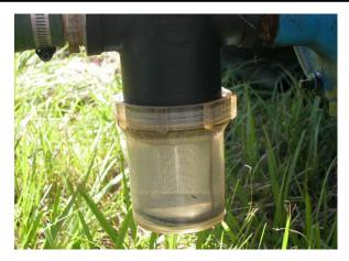
**Strainer.** Strainers like these allow a worker to see if debris has plugged a screen. Filters, like nozzles, should be checked regularly. Credits: UF/IFAS
