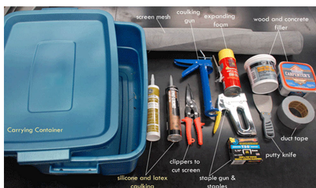
Figure 22. Equipment needed for bee-proofing. Credits: M. K. O'Malley, University of Florida
