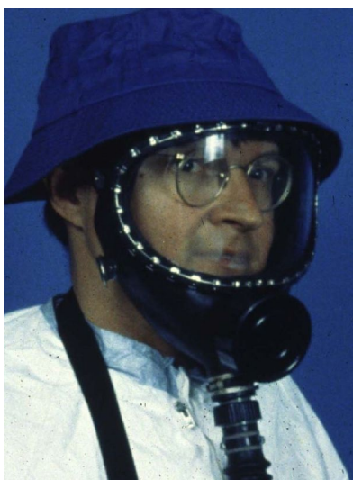
Figure 7. Full-face respirator provides eye protection
