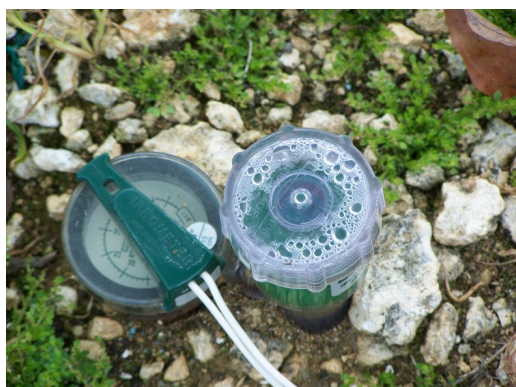
Figure 4. Switching tensiometer. Credits: H. Trafford
