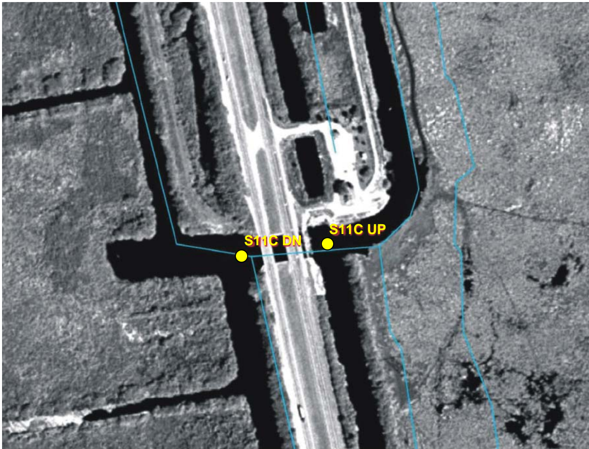
Figure 3. Example of head and tail gaging stations at S-11C. S-11C is a control structure in the levee dividing Water Conservation Area 2A from Water Conservation Area 3A-North.
