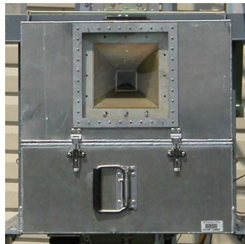
Figure 4 (b) and (c). The side view of the UFCMR showing the rotary system and the front view of the UFCMR showing the receiver antenna.
