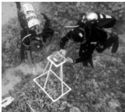
Divers using quadrat equipped with a camera to measure coral cover.
