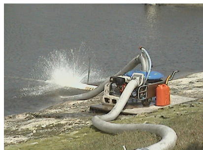
Figure 2. Fish pump operating from the outer-bank of the retention pond. Credits: Scott W. Grabe
