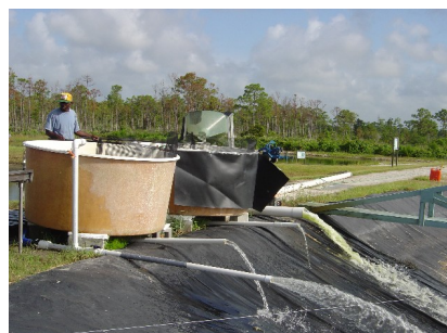
Figure 3. The arrangement of the green dewatering tower and the two round holding tanks on the levee. Credits: Cortney L. Ohs
