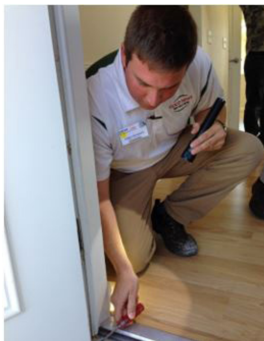
Figure 29. Probing and sounding door frame and door threshold during termite inspection exercise at UF/IFAS Extension program, Pest Management University.
