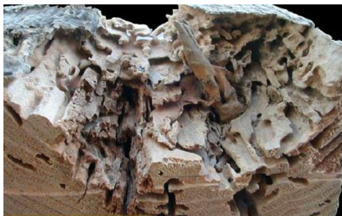
Figure 19. Neotermes jouteli (Banks) damage in 4-inch x 8-inch beam removed from a house in Ft. Lauderdale.
