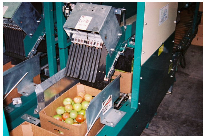
Figure 8. Shipping cartons are automatically filled by weight.
