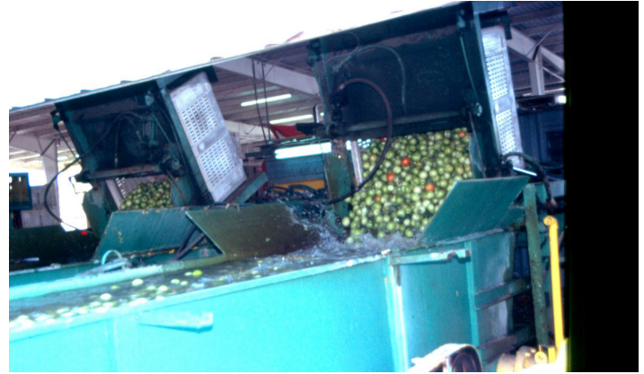
Figure 5. Field bins normally are emptied into a dump tank to minimize mechanical injuries.
