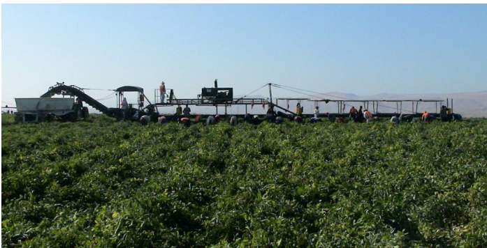
Figure 4. A mobile conveyance system increases hand harvest efficiency.
